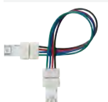
LEDFLEX IN RGB CONNECTION SET 300 92 93 05 4 x 0,35mm 2 / 150 mm SET OF 10 pcs
