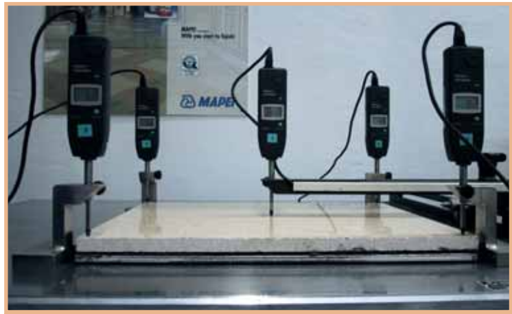
Fig.2 Bonding test with an adhesive
