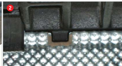
Align anti-shunt detail with recess
